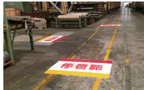
Intersection traffic control
