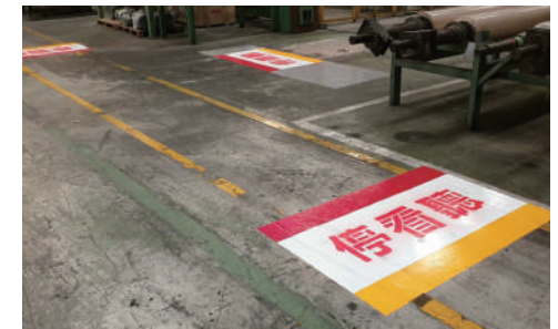
Intersection traffic control
